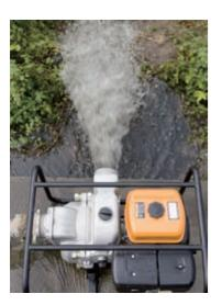
For those applications where large solids and debris are encountered, KNOXGEN offers a line of trash pumps designed to meet the infiltration of such debris. Deep impeller vanes and a large volute discharge opening can pass suspended sticks, stones and debris without clogging the pump or harming its components. Designed to be user-friendly, these self-priming pumps remain durable under the harshest conditions.
